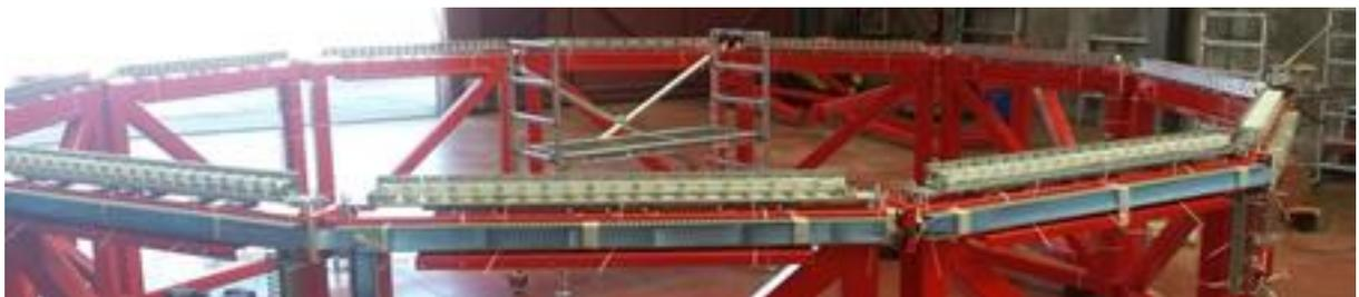
**Figure 2:** Tomography system for imaging CO<sub>2</sub> concentration distribution at the exhaust of an aerospace engine. The 12 optical alignment plates and individual launch/receive optical elements are visible on the ring's segments.
